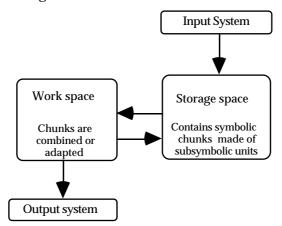
This message passing system enables different structures to be used. A chunk may constitute an "If <condition> then <conclusion>" rule, or a "<stored input pattern> <conclusion>" example.
